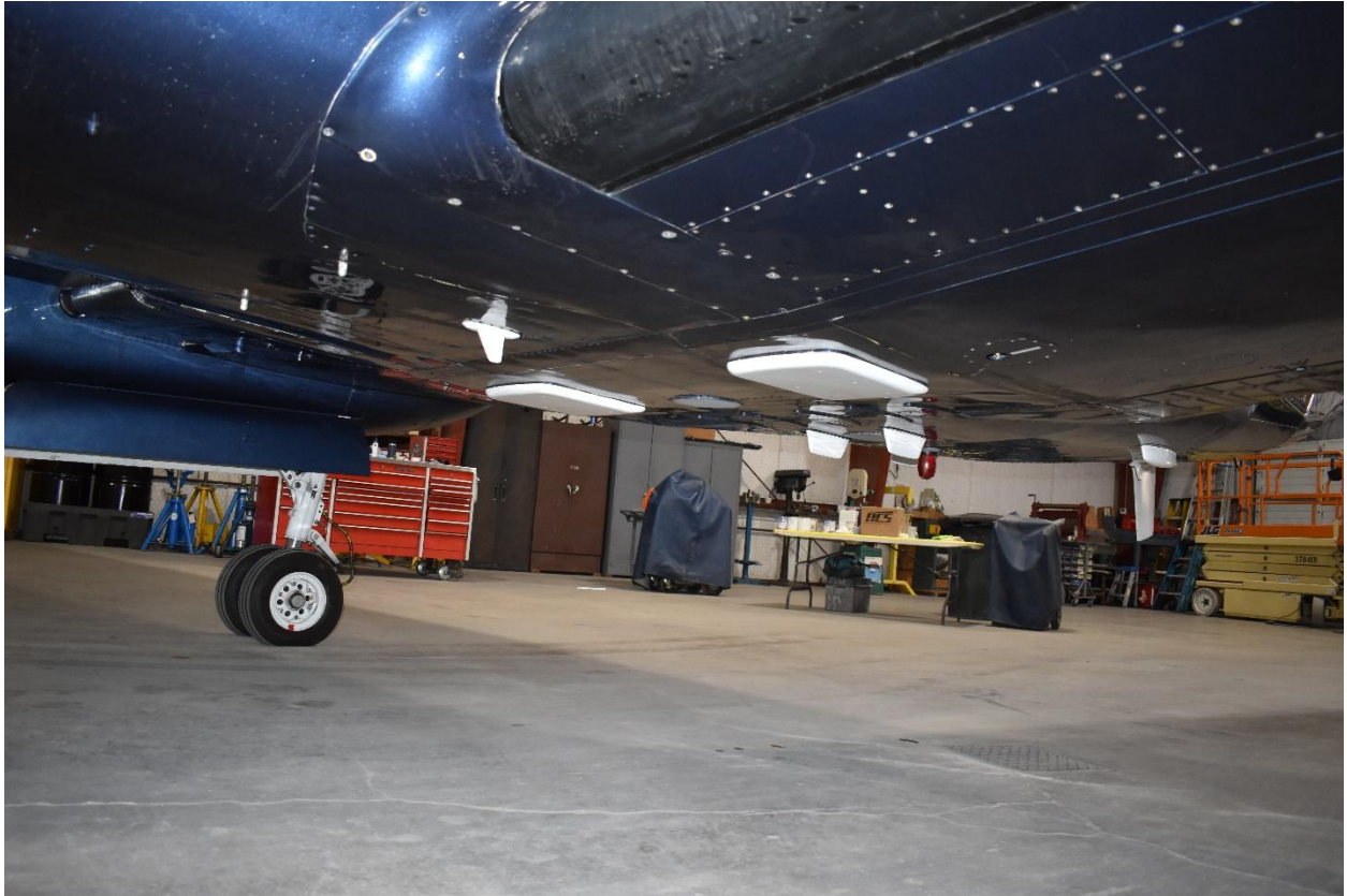
Inboard lower left-wing fasteners without paint treatment
