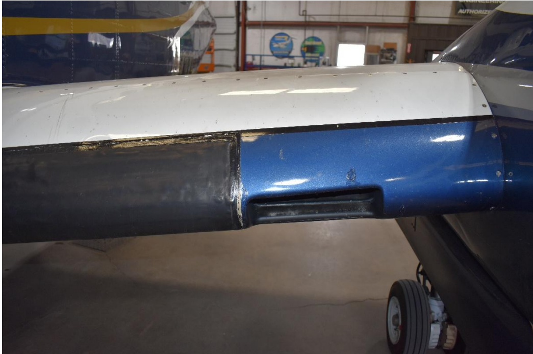
Inboard lower left-wing fasteners without paint treatment
