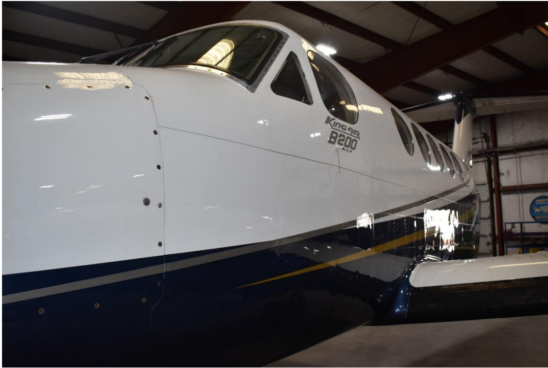
Gloss Paint Treatment – fasteners with out paint from wear
