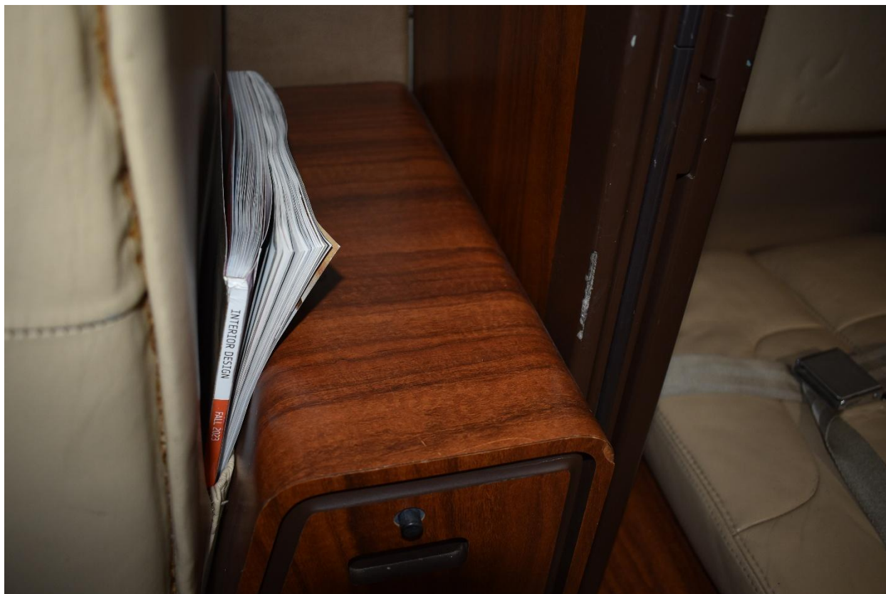
Storage cabinet with chip in the lamination on the aft corner edge
