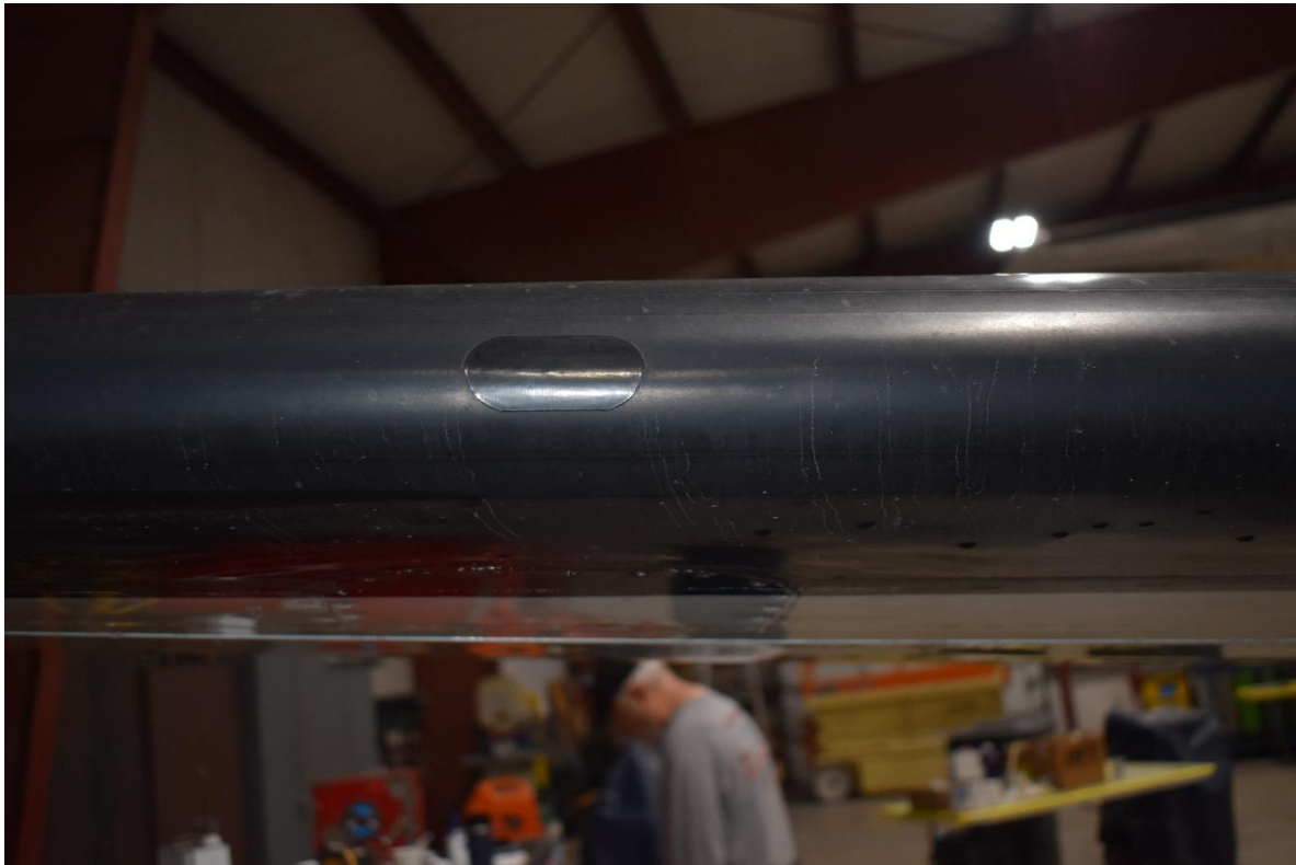
Deice boot repair
